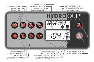
**Default System Operation:** When power is applied, or there is a temporary loss of power, the system will initiate its default programming. The filter cycle will begin 24-hours after the system has been powered up. The filtration cycle will be active for 1-hour and will repeat every 24-hours. The temperature will be maintained at 95°F.
